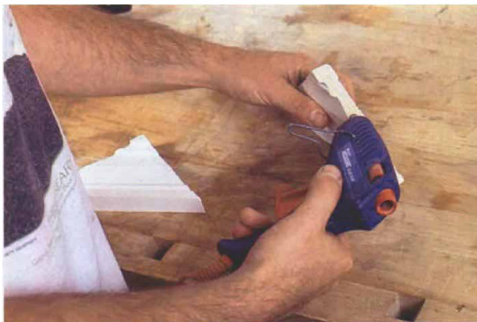
Melt, aim, shoot. This trigger-fed gun squeezes a hot bead of glue from its tip. The glue sets quickly as it cools, making it great for sticking together a prototype to see how it'll look.
