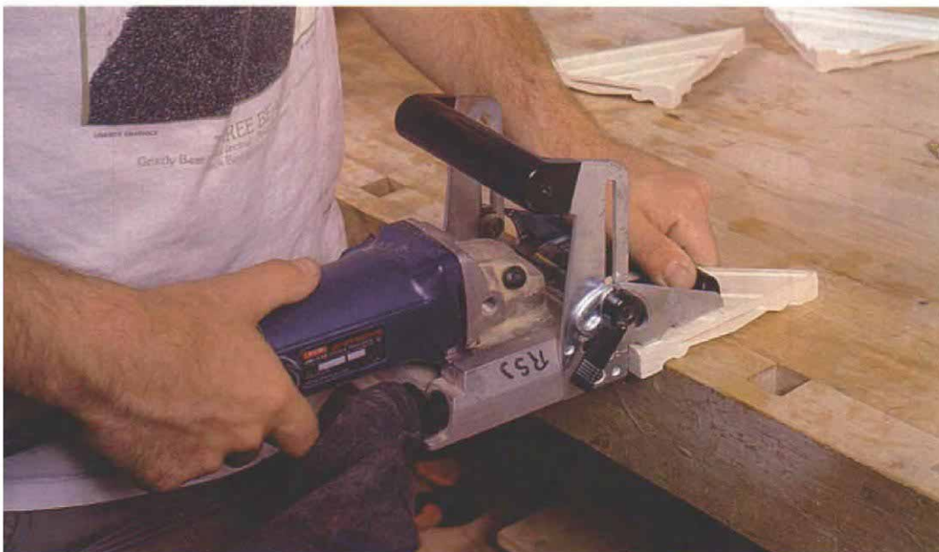
Another use for the biscuit joiner. After carefully cutting and aligning the four triangles, biscuits are inserted in slots to keep the joints tight through all of New England's weather cycles.
