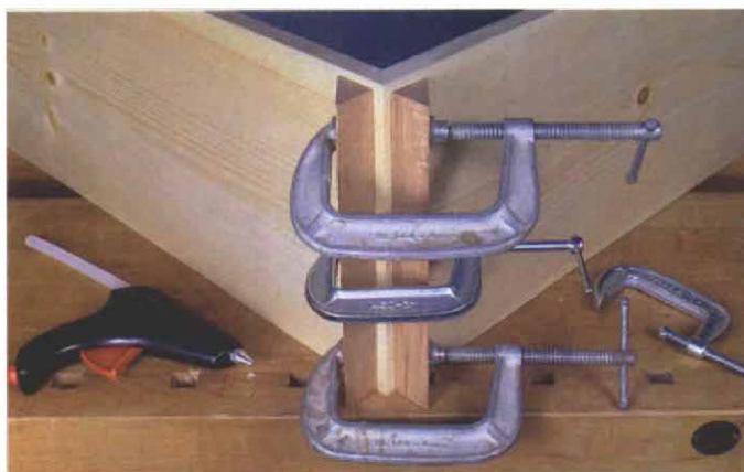
Temporary clamping blocks. To clamp miterjoints, triangular clamping blocks can be made with hot-melt glue. The blocks can be easily removed later without damaging the mitered pieces.
