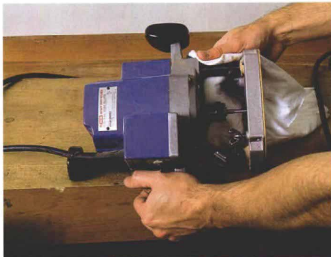
Clean plunge posts. Wipe posts with a dry cloth but avoid oil-based lubricants. They attract dust and may foul the plunge mechanism.
