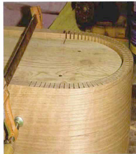
Perfectly kerfed. Kerfing begins before the form bends to eliminate tension in the riser stock; well-kerfed wood wraps around the form like a piece of paper. Here the kerfed stock is temporarily clamped so that the other bullnose end can be marked for kerfing.
