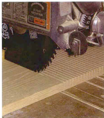
Kerfing with a radial-arm saw. Kerfs are crosscuts that don't cut completely through the stock. Here the kerfs are \frac{3}{8} in. o. c., and the face is \frac{1}{16} in. thick. Although the author used a radial-arm saw, a circular saw, a straightedge and elbow grease will yield the same results.
