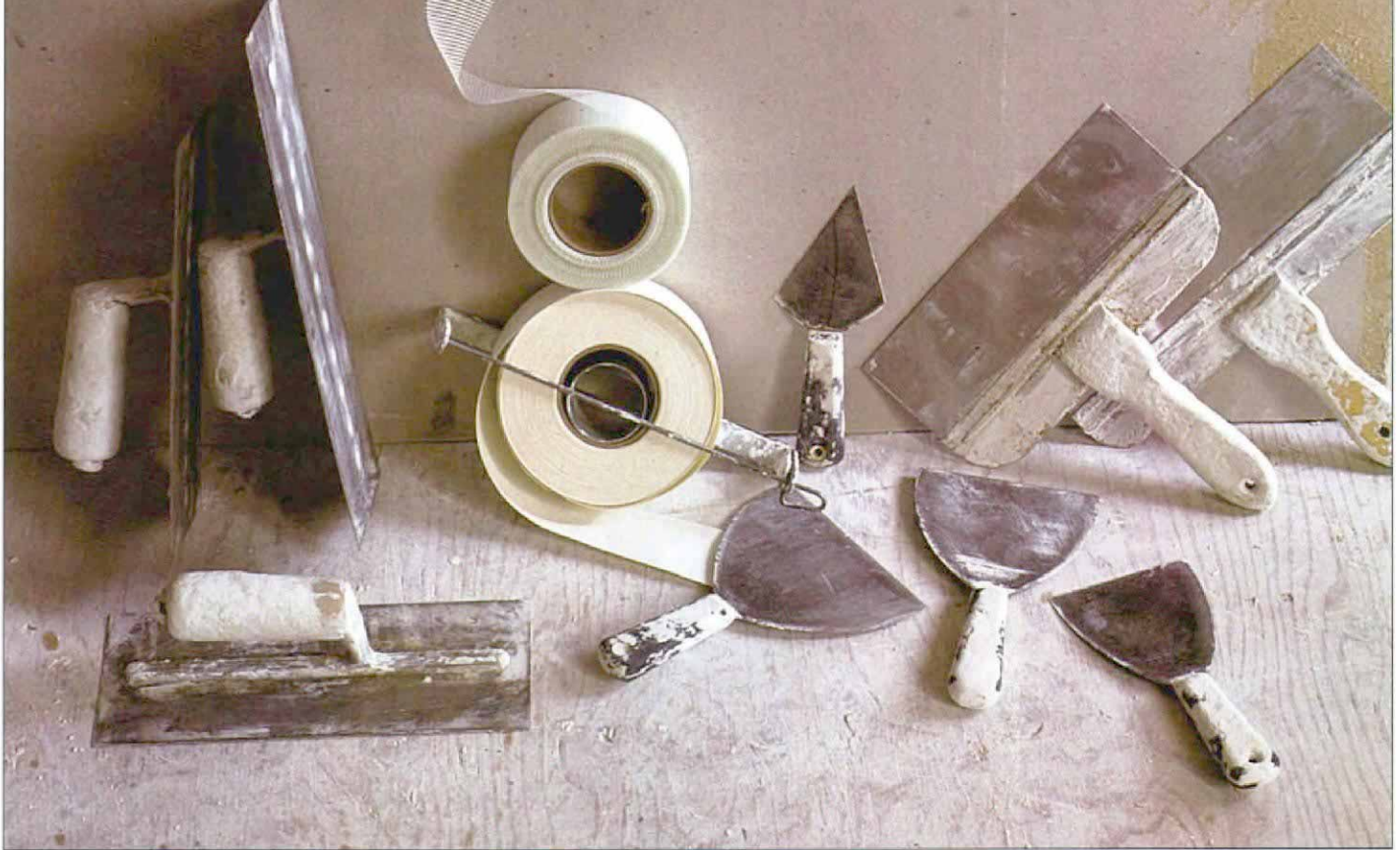
A tapers' toolbox. Left: a set of drywall trowels. Center: rolls of fiberglass and paper tape. Right a sampling of tapping knives.
