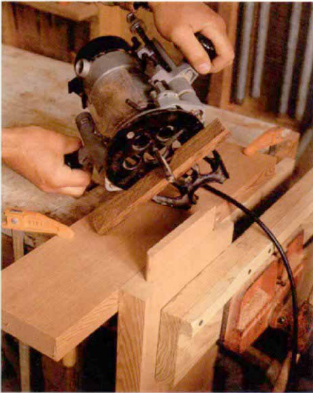
Loose tenons. While interior doors can be joined with dowels, the abuse experienced by exterior doors requires the broader gluing surface of a spline, or loose tenon. The spline should be a bit narrower than the mortise to allow the pieces to be adjusted during glue up.
