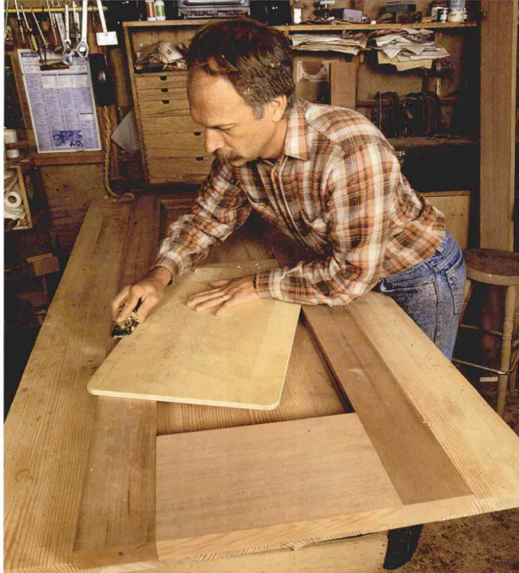
Radiused and beveled core panels. Cutting the slots in the frame with a router makes for rounded corners. The plywood core panels need to be rounded to match. The panels will fit into their slots easier if their edges are beveled with a hand plane.
