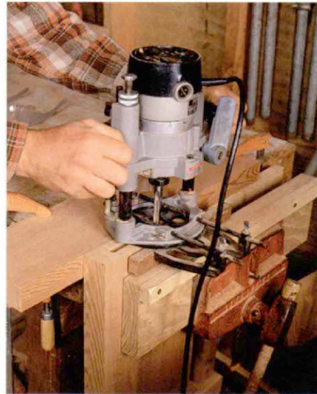
Routing a mortise. A bench vise is the best tool for securing a rail or stile as it is routed. Here, the bit is guided by a fence attached to the router's base. A block clamped to the bench provides a broad surface for the plunge router to ride on.
