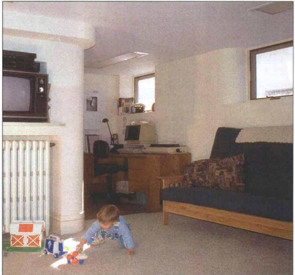
**Kid-friendly.** Curved corners add comfort and safety to a room for children. Bending plywood creates these corners, which are spackled, taped, skim-coated and painted exactly like drywall.
