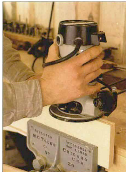
Cutting the mortise. The mortise in the head casing is cut with a fence-guided router and a 1/4-in. carbide spiral bit. The first pass is made on one side; the second, on the oilier.
