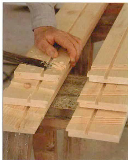
Removing the waste. The author quickly pares away waste with a sharp chisel. Because the orientation of the 12° cuts defines the handedness, left and right jambs are needed for each window.
