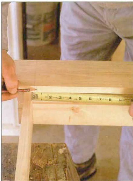
Tenon layout. Side casings are laid out for the joint that connects the head and side casings. The left line is the total length of the casing. The other line is the shoulder of the tenon.
