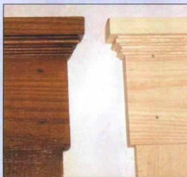
A table saw and a shaper were used to make ash molding (right) that matches the original chestnut trim (left).
