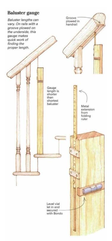
Some staircases call for square-ended balusters that fit into a groove plowed into the underside of the handrail. In an ideal world all the balusters for a given position on each tread would be the same, and you could just go along and cut sets of short and long balusters. For various reasons, though, baluster lengths can vary as much as  $\frac{3}{16}$  in.
