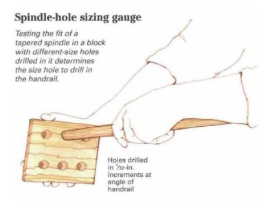
The diameter of the top, or thin end, of a tapered spindle can decrease as the spindle gets longer. Therefore, the hole drilled into the handrail for the back spindle on a tread can be smaller than the hole for the front baluster.
