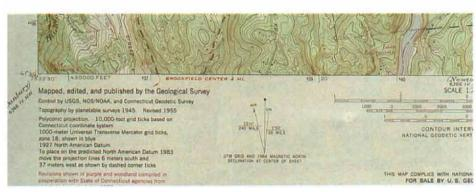
Topographical map shows declination. The U.S. Geological Survey prints maps that show the lay of the land. At the bottom margin there are three north bearings: magnetic north, true north and grid north. Magnetic north is compass-needle north, but it won't be helpful for solar siting, which calls for true north, indicated by the star. The difference between these bearings is the declination; in this case it's 13.5°.
