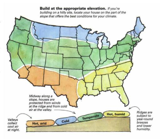
Cold air flows downhill. Cold air is heavier than warm air, so at night cold air travels downhill along natural drainages and depressions.
