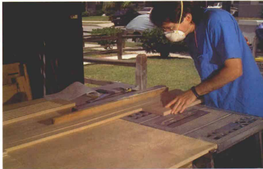
Cut multiple flutes without moving the fence. The pilaster faces were fluted on a router table by registering them against 1-in. MDF strips instead of directly against the rip fence. After each pass, a strip is removed; the rip fence is not moved.
