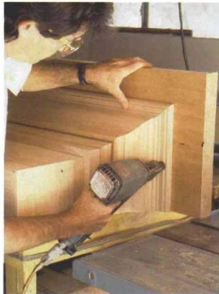
Fastening the crown. Once the shelf is fastened to the frieze box, the crown molding is applied. The front piece goes on first, and the mitered ends are glued and nailed in place.
