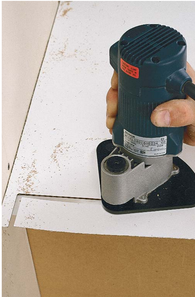
An offset base allows you to get close to vertical surfaces. Handy for such jobs as routing sink openings and trimming the top edge of a backsplash, an offset base is available separately or as part of a trimmer kit from DeWalt, Porter-Cable and Bosch.
