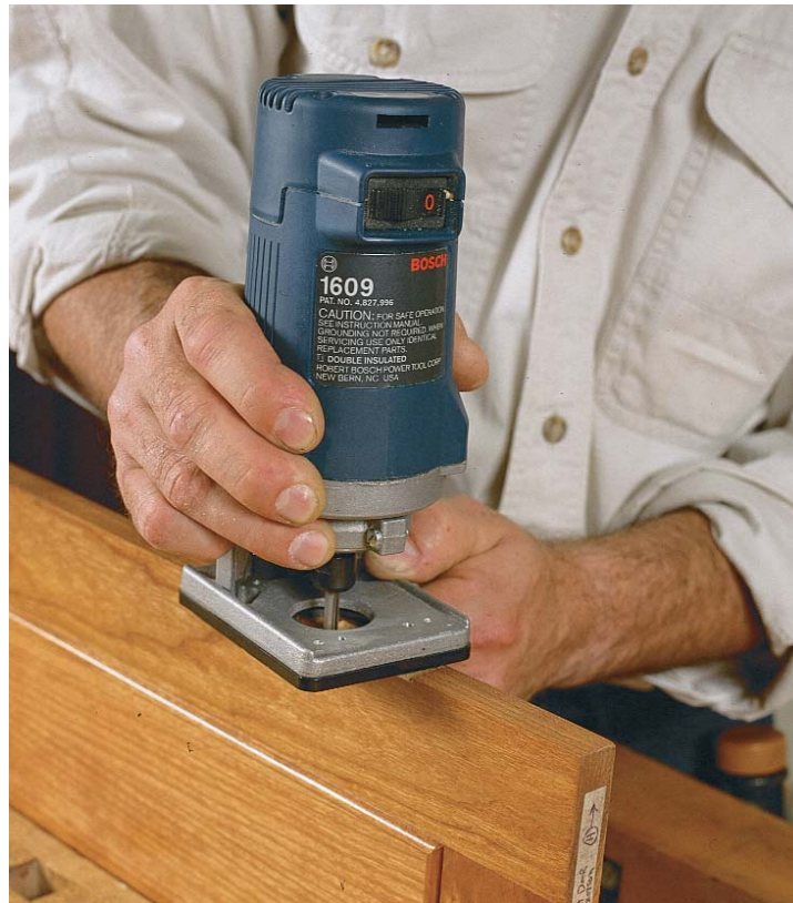
Easier to handle than conventional routers. Freehand mortising a cabinet-door edge for hinges is relatively simple with a 1/4-in. straight bit chucked in a laminate trimmer.
