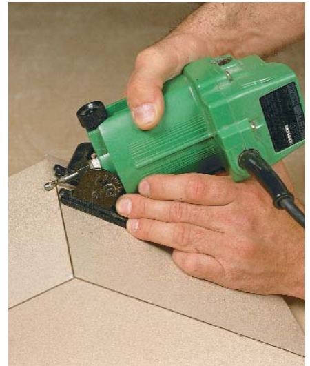
Tilt base is standard on the Hitachi. When trimming edges that join at angles other than 90°, use a tilt base. Most manufacturers offer them as accessories. Tilt bases also allow the trimmer to reach close to a vertical surface, but you can't use a bearing bit. You'll have to use a self-pilot bit such as the one shown here.
