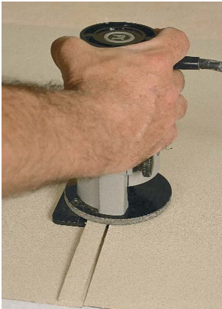
Make perfect seams. With an underscribe-trimmer base, you can mirror-cut seams in plastic laminate using the bottom piece's factory edge as a guide. The trimmer bit cuts the top piece only.
