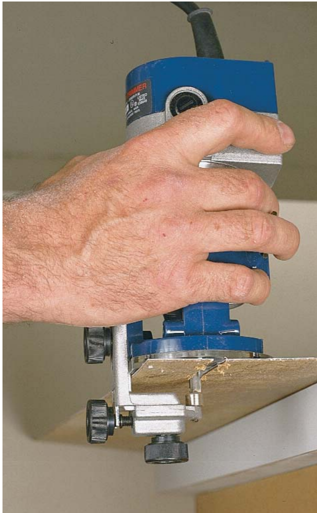
Skis are a unique DeWalt accessory. Two 3-in. lengths of plastic screwed to the trimmer base allow the bit to straddle the hardened adhesive ooze along a solid-surface countertop seam and rout the adhesive flush to the surface.
