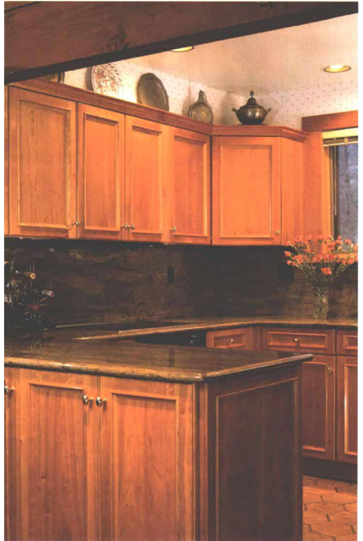
Frame-and-panel doors provide a traditional look. These cherry cabinets with a lacquer finish employ cup hinges, so the doors hang on the cases instead of from a separate frame. The moldings that frame the door panels emphasize the traditional appearance.
