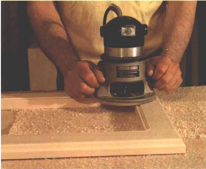
A rabbeted edge to hold the panel. Instead of a groove to house the panel, a rabbet creates a ledge against which the panel is seated. Rabbeting is simpler because it allows you to assemble frames first without the panel to complicate assembly. The rounded corners are squared with a chisel.
