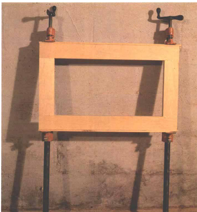
Assembled frames are clamped with pipe clamps. It takes about a day for the frames to set up. Pressure blocks prevent clamps from damaging the frames. Clamps must be centered through the thickness of the frame, or they may pull the frames out of flat.
