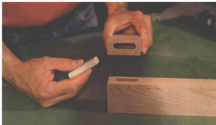
Door-frame joinery features a simple, quick loose-tenon joint. A loose tenon ripped from solid poplar fits into mortises in the stiles and the rails. Mortises are cut with a ⅜-in. straight bit in a plunge router.
