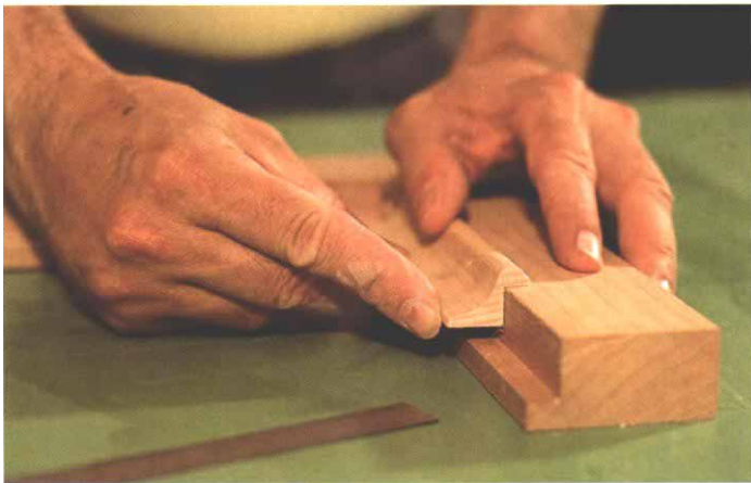
Panel molding is rabbeted to fit over frame. The depth of the rabbet in the frame depends on the thickness of the panel plus the seated depth of the panel molding. The panel molding holds the panel in place.
