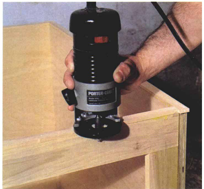
Here, edging is trimmed on the case's top frame. After the edging is glued and nailed in place, the overhanging edges are trimmed with a trimmer bit in a router. Edging tears out easily, so the first few passes should run right to left; the final pass runs left to right.
