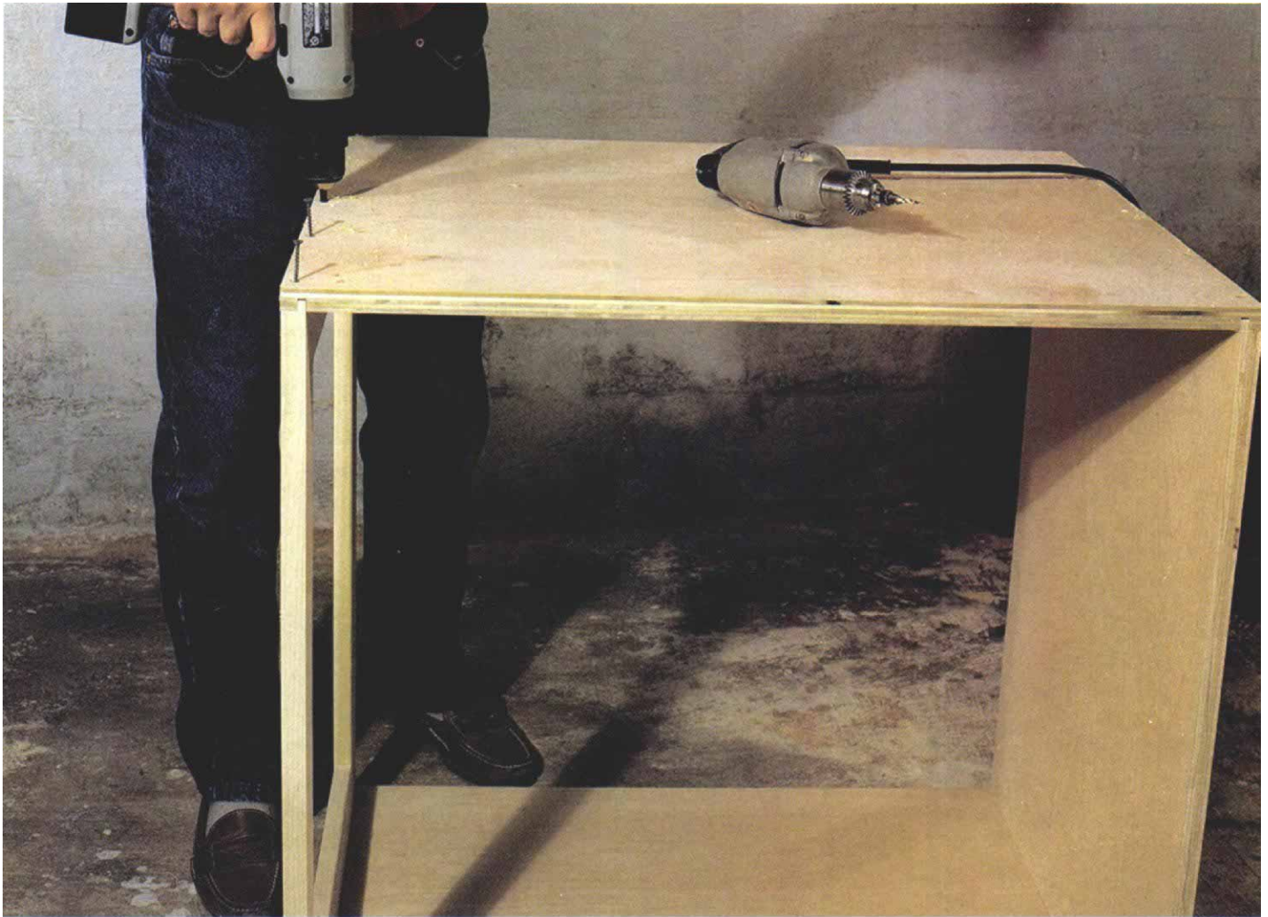
Cases are assembled with glue and screws. With the case lying on its side, the side panel is screwed to the top frame. Tongues in the top frame and the bottom panel interlock with dadoes in the side panel. Small gaps between the tongues and the dadoes allow for glue runout.
