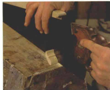
Run mitered returns long; trim them with a handsaw. The author uses one hand to hold the handsaw while he makes the cut.
