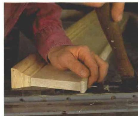
Nail the head moldings on a flat surface. To align the pediment's components, the author nails the pieces together on a flat surface.
