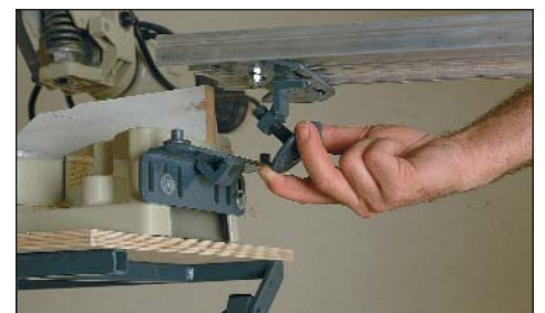
A saw stand that stands out. AD&E's SawHelper combines many top features: It is lightweight, is easy to carry and set up, and comes with extension wings and a calibrated stop. The bracket (photo below) lets the stand's wings attach to the saw for precise alignment every time the stand is set up.
