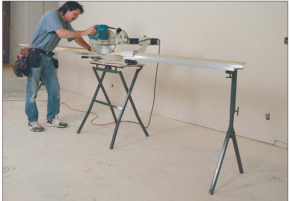
A saw stand that stands out. AD&E's SawHelper combines many top features: It is lightweight, is easy to carry and set up, and comes with extension wings and a calibrated stop. The bracket (photo below) lets the stand's wings attach to the saw for precise alignment every time the stand is set up.
