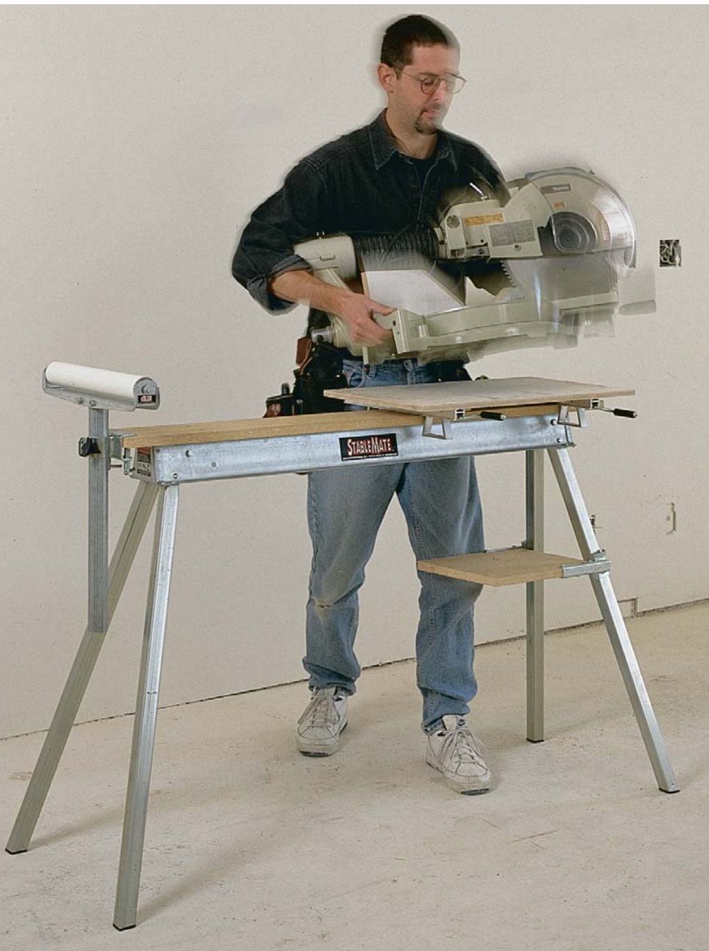
Portability, productivity and comfort. Stands in a range of shapes and configurations provide workers with comfortable platforms for chopsaws. Iowa Manufacturing's StableMate (the sawhorse) and Wedge (the saw platform) fold for easy portability, but its rollers offer minimal work support.
