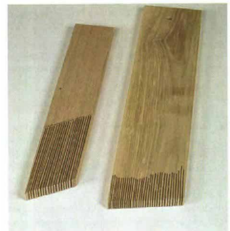
Kerf length affects stiffness. Longer kerfs make more flexible feathers, which make it easier to push bowed stock past the cutter. Different angles allow each featherboard to be clamped to a different area of the table.
