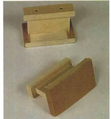
Sandpaper provides grip and is replaceable. The author made his own push blocks easily and cheaply from three pieces of scrap screwed together. The blocks are made in pairs, one for each hand.
