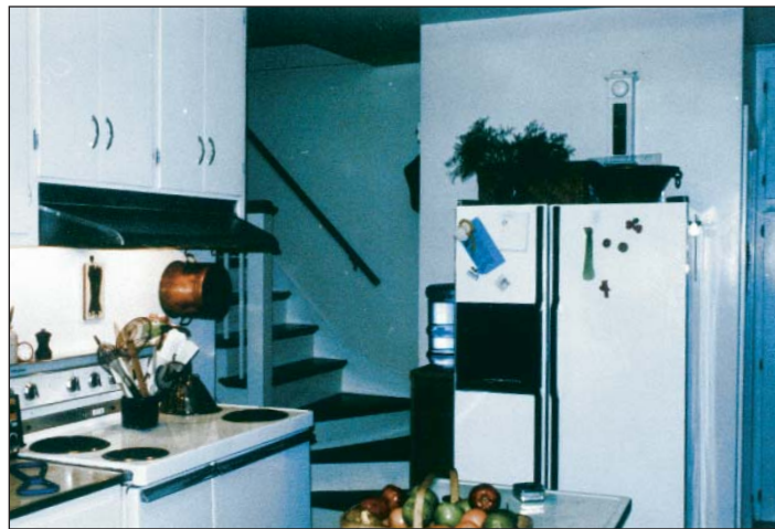
Same place, before and after. The cramped original kitchen (above) needed a more efficient use of floor space. Reorganizing the original pantry, moving the pantry wall back and recessing the refrigerator into part of the old space eliminates much of the congestion in the new kitchen (facing page). The custom-built, quartersawn oak worktable functions like an island but takes up less room.
