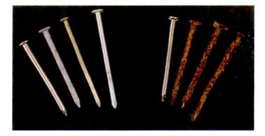
Ring-shank nails won't do this. After years of moisture cycling, smooth-shank nails work loose and pop up. Deformed-shank nails stay put. Stainless steel lasts
