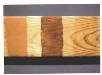
the first coat is dry, it seals the surface, and the second coat forms a film.
