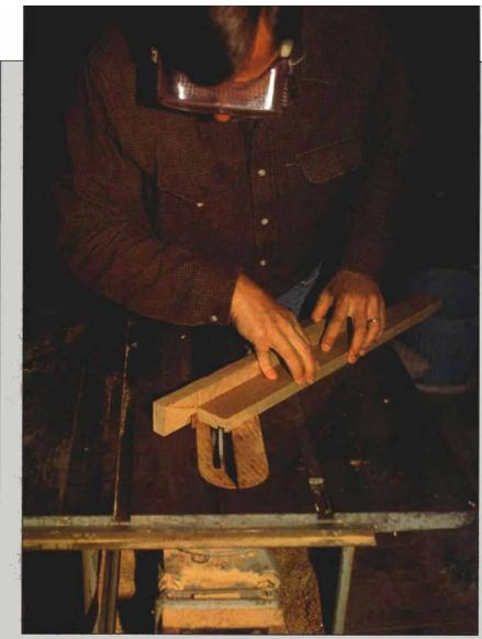
The trick to properly spaced slots is an indexing stick. The author attached the indexing stick to the miter fence on his table saw and set the small index pin, which is visible at the left of the stick, into the last slot cut, thereby perfectly aligning the piece for the next dado cut.
