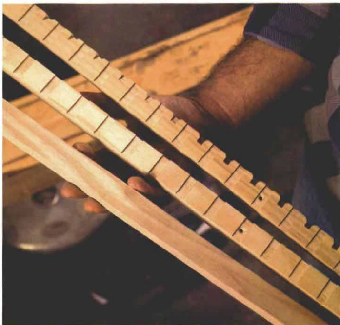
Finally, the cross braces are sized and kerfed. Shown here are the three stages of the cross braces used on the dish rack. These pieces will go on the back of the rack. The dadoed slots between the curved kerfs hold the vertical dividers and the cup hooks.
