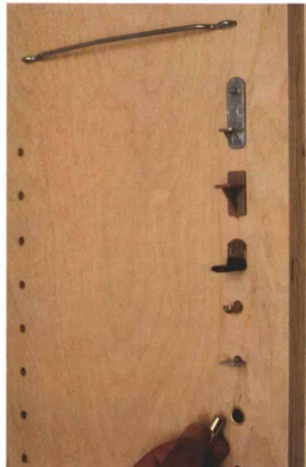
Shelf pins are inconspicuous. Shelf pins are less visible than shelf standards. Top to bottom: wire clip, which hides inside a groove at the end of a shelf; spring-loaded locking clip that prevents shelves from sliding or tipping; plastic clip; cushioned metal L-support; ornamental solid-brass pin; zinc-plated steel paddle; "library" pin with sleeve.
