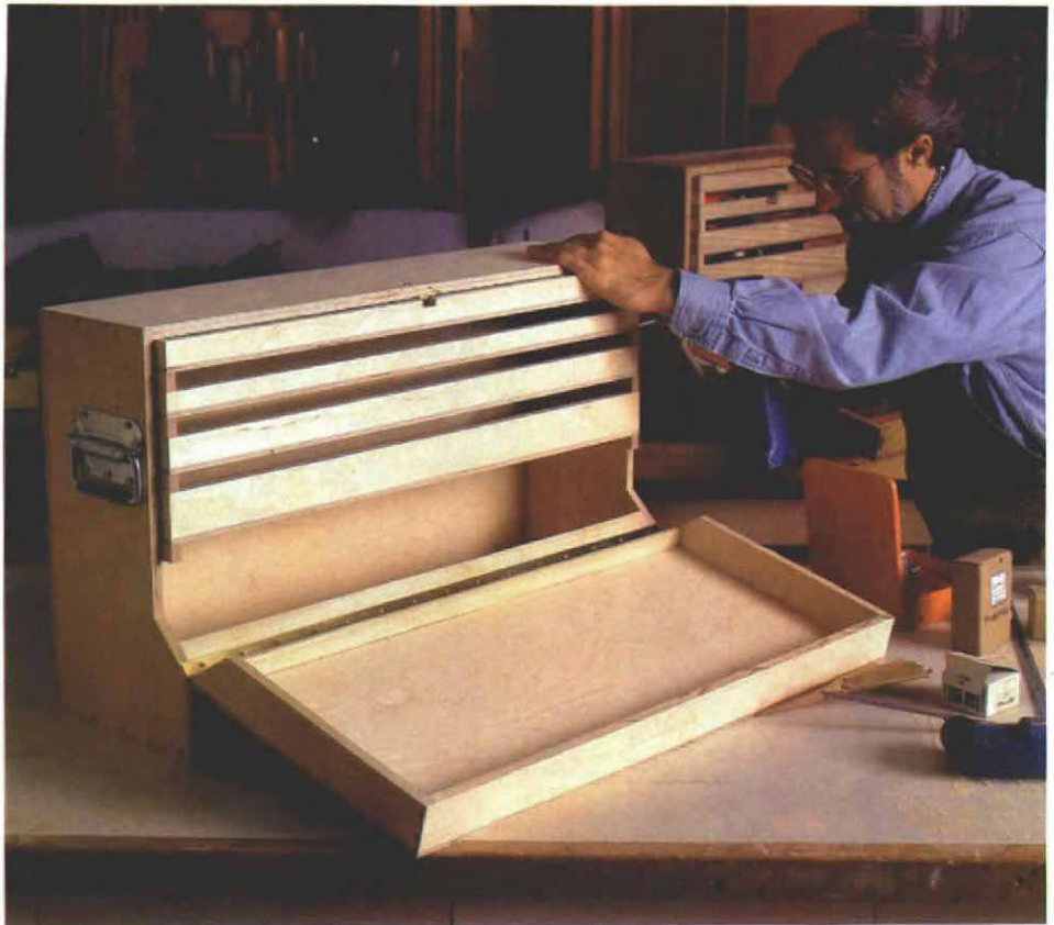
A piano hinge links box and lid. The bottom of the lid is lopped off at a 45° angle and is reattached to the box to become the mounting block for the lid's hinge. For this box, the author affixed bail-type handles to the box's ends.
