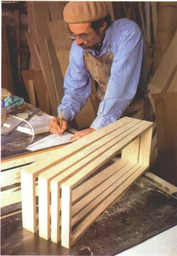
Four drawers from a single box. A quartet of different-depth drawers are ripped to width on the table saw from a single box. Glued and nailed plywood bottoms, ¼ in. thick, complete the traylike drawers.
