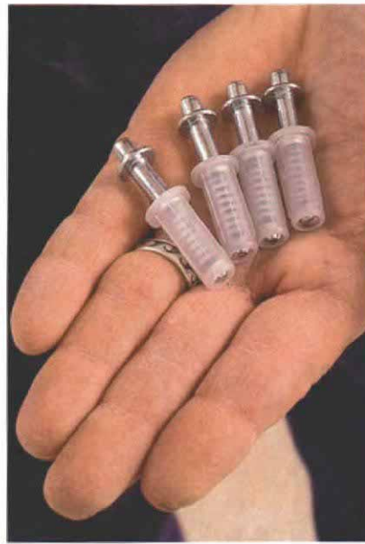
13, 14. The doors swing on pins. At the top, each door has a spring-loaded pivot pin (photo left) that slides in the door track. At the bottom, the door closest to the jamb has an adjustable pin that fits into the jamb bracket (photo above).
