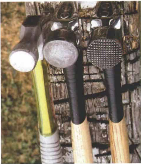
The many faces of hammers. The hammer on the left has a standard smooth face for driving finish nails. The middle hammer has a face with a sandpaper texture that helps to keep the hammer on the nail, while the milled face on the right hammer grips the nail aggressively for framing.
