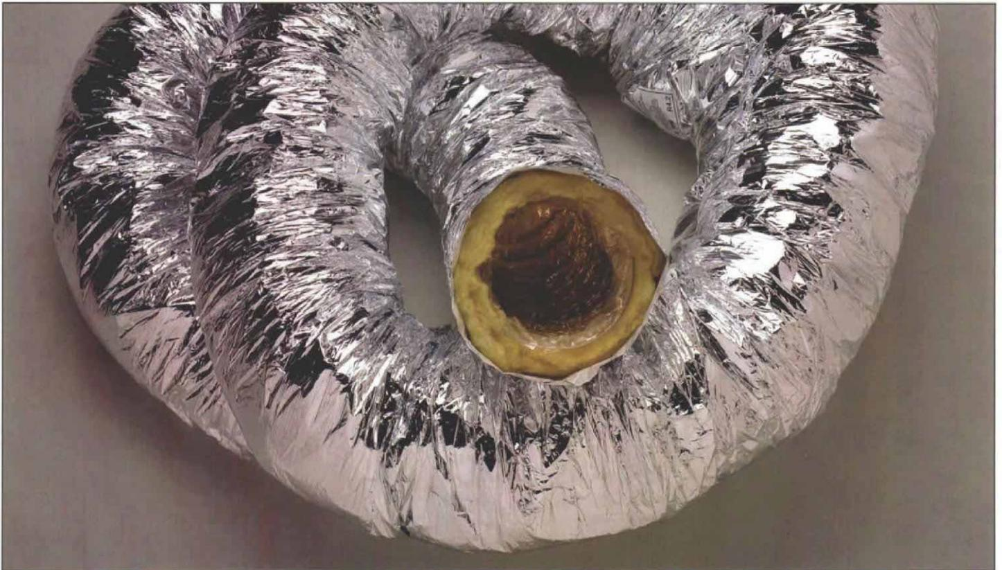
**It bends easily, but at a price.** Flexible ductwork, such as this insulated, foil-covered duct, is good for getting up and over a joist or around a corner. However, the ridges inside the duct slow air so much that it shouldn't be used for straight runs.
