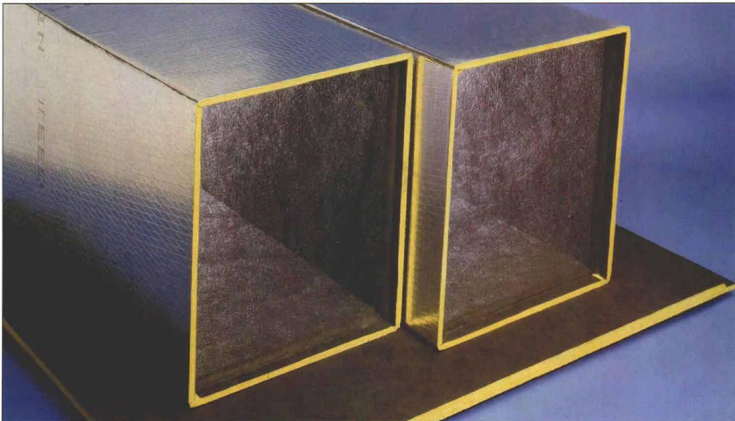
**Duct board is rigid fiberglass faced with foil.** Preinsulated ducts made of duct board are generally leakier than rigid-metal ducts and puncture more easily. The seams are prone to failure unless assembled under clean shop conditions.
