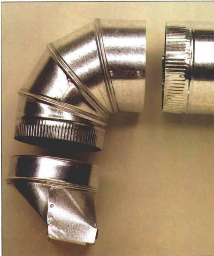
**The best bet for ductwork.** Round, rigid-metal ductwork is the best choice for delivering air throughout a house. However, these fittings—a 90° elbow and a round-to-rectangular transition—create resistance to the airflow and should be used judiciously.
