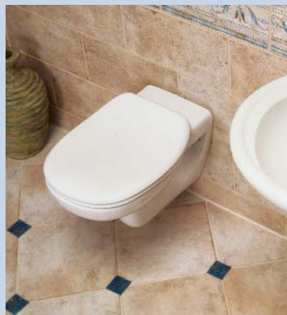
No floor drain required. This wall-mounted toilet, the Kimera by American Standard, discharges to the rear so that no floor drain is needed. The rear-discharge feature is useful for remodels, where installing a floor drain would be impracticable. Photo courtesy of American Standard.
