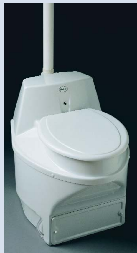
An all-in-one composting toilet. This self-contained BioLet composting toilet contains an automatic mixer, a heating element to accelerate composting and a fan to draw odors up the vent. Photo courtesy of BioLet.
