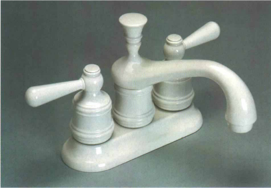
A 4-in. center-spread faucet takes up little room. With the valves and the spout mounted together in a single base, this Moen faucet measures 4 in. from handle to handle. List price: about $152.
