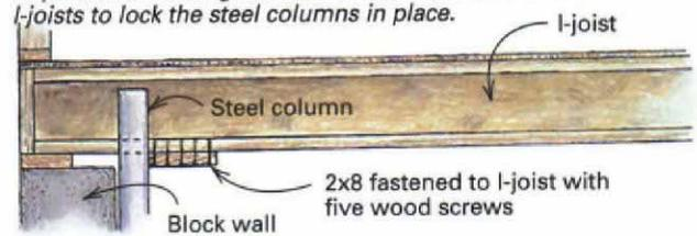
If the joists are parallel to the foundation wall, the blocking must be braced as shown below. I-joists require the addition of diagonal bracing.
