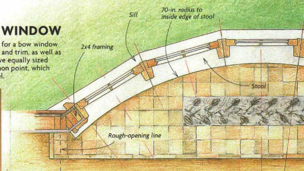
Radial lines for equally sized window sash
