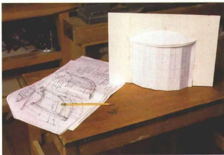
**A paper model proves a point.** The author was convinced the roof would be a section of a sphere—until he made a paper model. He had to agree with his building partner that the roof was actually a conical section, much easier to frame and sheathe.
