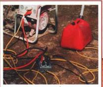
**Too many power tools can overload an extension cord.** When a wire is overloaded, its insulation can melt and short-circuit, sparking a fire in the surrounding area.
