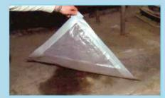
The poly test determines if drylooking masonry is passing water. Left overnight, a plastic sheet will cause misleadingly dry-looking concrete to dampen visibly.
