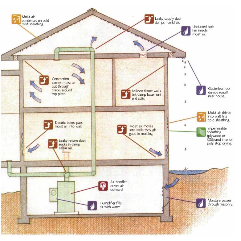
denses on every cool surface, and mold flourishes. Although this procedure may be a code violation, experience has shown me that permanently blocking all vents in foundation walls is a sure way to save sills and floors from condensation-induced rot. If restricting air to combustion appliances such as a furnace or water heater isn't a problem, I insulate the walls with extruded foam and seal perimeter air leaks with polyurethane foam.
