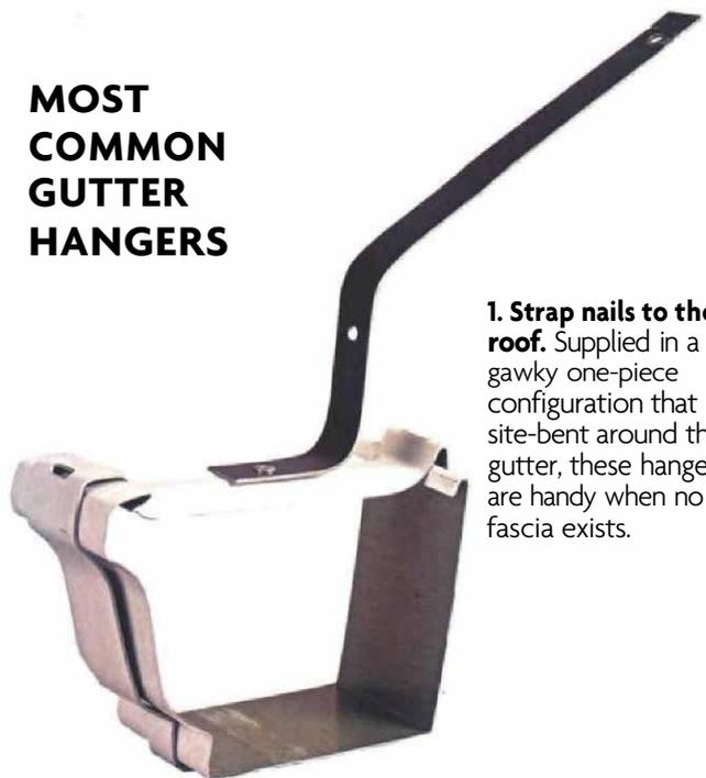
**1. Strap nails to the roof.** Supplied in a gawky one-piece configuration that is site-bent around the gutter, these hangers are handy when no fascia exists.
