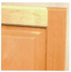
A step up in a wood design. This maple KraftMaid door has a solid-wood raised panel and a smoother, less brassy finish than the door on a budget cabinet. The cope-and-stick joinery is essentially the same. The color and figure of the maple pieces used in both the panel and the frame are not perfectly matched.
