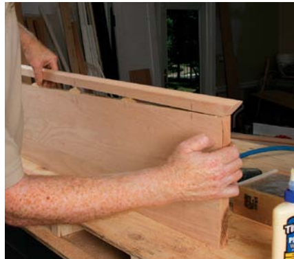
Put the treads back together. Biscuits align the top of the nosing and tread. Pocket screws from below draw the nosing and tread together, clamping them as the glue sets. Stagger the two so that the screws bite into the oak, not the biscuits.
