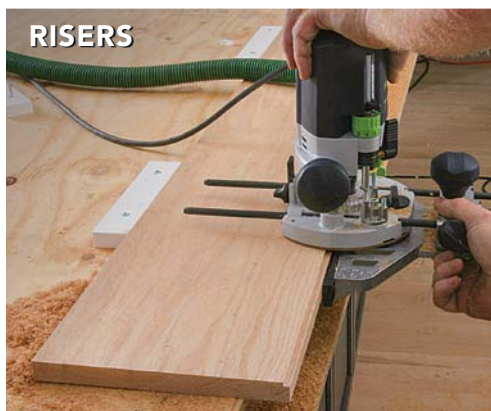
Machine the treads and risers. Rabbets in the risers slot into dadoes in the treads. This ensures tight joints and corrects any bows in the risers when they fit into the tread dadoes.
