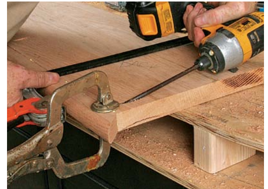
Put the treads back together. Biscuits align the top of the nosing and tread. Pocket screws from below draw the nosing and tread together, clamping them as the glue sets. Stagger the two so that the screws bite into the oak, not the biscuits.
