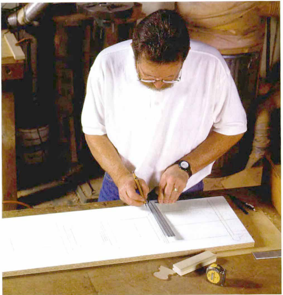
Full-size drawing makes design an easier process. On a piece of scrap melamine, the author draws a detailed elevation and cross section of the newel, which allows him to plan carefully and to give the client a good indication of the newel's proportions.
