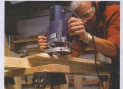
**Two routers make quick work.** The first has a bearing-guided straight bit and removes most of the stock up to the template edge. The second is also bearingguided, and it miters the edge.
