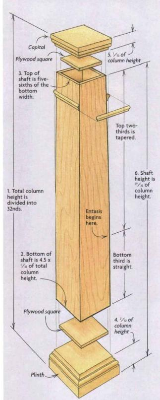
**Proportioning a Tuscan column.** Start by dividing total height into 32nds. Using a 96-in. tall column as an example, the math below follows the steps shown in the drawing above.
