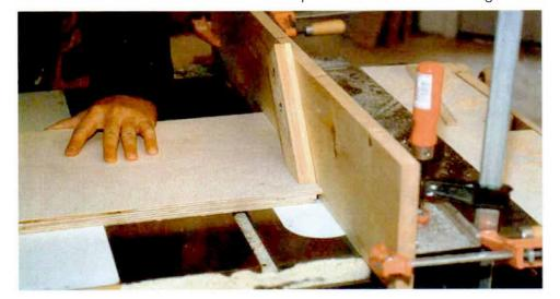
**Cutting the tongues.** A featherboard attached to an auxiliary fence makes the process safer and the tongues more consistent in thickness.
