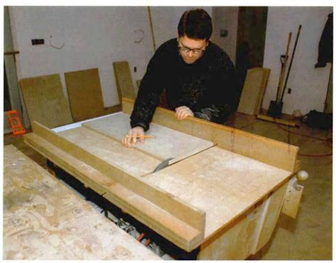
**It's safer with a cutoff box.** A table-saw cutoff box ensures that cabinet parts will be square. When working with Baltic birch, don't assume that factory edges are square.
