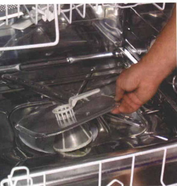
Removable filter can save a dishwasher. European-style dishwashers have mesh filters that can catch harmful debris such as broken glass before it can damage the inner workings of the machine.
