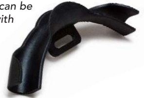
Nylon grommets protect the tubing. Available from most distributors, grommets are cheap insurance for tubing that passes through sharp-edged steel or wood studs.
