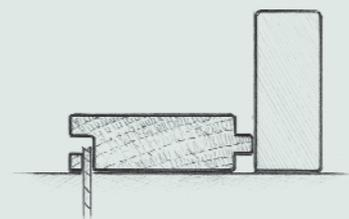
Remove the bottom of the groove from the new board on a tablesaw. This removal allows the new board to slip over the tongue of the adjacent floorboard.
