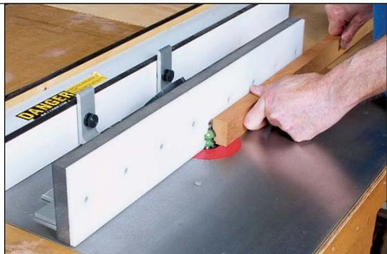
Although designed to make base-cap molding, the bit pictured at right is similar to the one used to create the band molding for the pine sample on the facing page.
