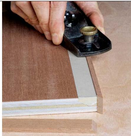
**A mitered return** cut from the same piece of plywood stock eliminates color-matching problems when staining. Small returns such as this one are often just glued in place.
