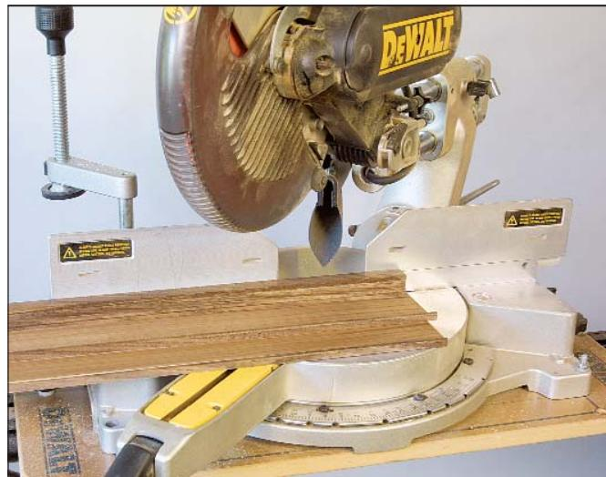
Rather than running six individual pieces of trim around a door or window, you can glue, align, and clamp them to create a composite molding, which you then can miter as a single piece. To avoid dangerous shrapnel and to protect the sawblade, be careful not to cut through any nails.
