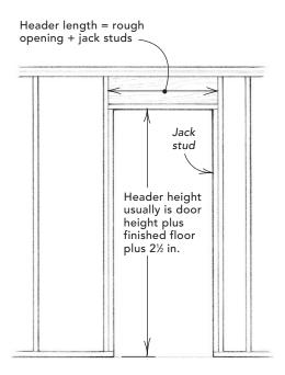
are a nonstandard height, you'll need to figure out the header height. Finding the height of the bottom of the headers above the subfloor is a matter of adding up the door height, the thickness of the finished-floor materials, and 2½ in. (to allow space for the head jamb and airspace below the door). There are exceptions. Pocket doors typically require a rough opening at least 2 in. higher than a standard door. Windows may include arches or transoms, which affect the rough opening's height.
