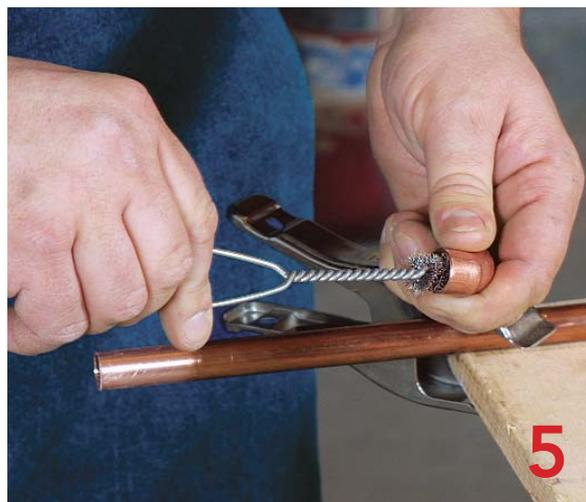
**Scour the pipe and the fitting.** To remove oxidation (tarnish) that would impede the bond between solder and copper, polish the outside of the pipe with a length of emery screen (photo left), and scrub the inside of the fitting with the brush (photo right). Clean both surfaces until they shine like a brand-new penny.
