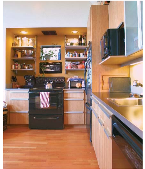
Adding space on a tight lot. In the addition's second floor, the author was able to incorporate a bump-out that hung out over the setback and made space for the stove and the cabinets. Photo taken at D on floor plan.
