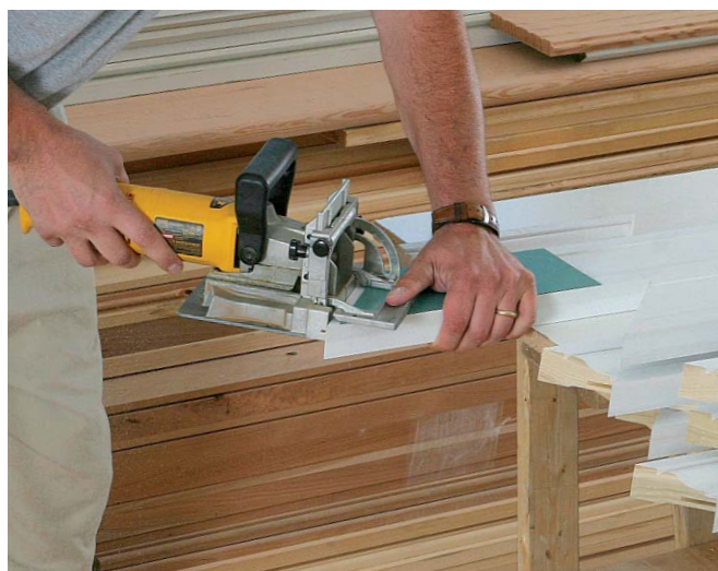
Slot all the miters at once to save time. After the stock has been cut to a rough length and mitered, the mitered ends are slotted for biscuits. To speed the process, each piece is partially pulled from the pile and slotted from the back; the miter's short point is used as the biscuit joiner's reference point.
