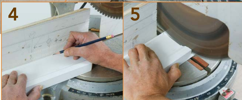
Mark the length, slide it over, and make the cut. With the miter already cut, the author can register a piece of the casing's miter against the stop block, transfer the correct measurement for that particular piece, then slide the piece toward the blade and make the square cut.
