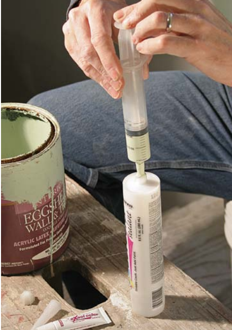
Add paint to the caulk tube. Measure out the specified amount of paint with the supplied syringe, then cap and shake.
