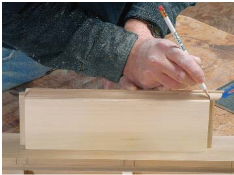
No measuring needed. The most accurate way to cut the stop is by marking it in place on a stile. The only measuring so far has been for the spacing of the muntins.
