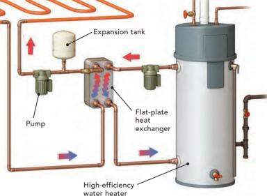
CONDENSING BOILER WITH INDIRECT HOT WATER
