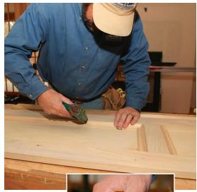
Add the inside molding after the plywood is attached. I glue and staple 1/4-in. plywood directly to the back of the frame, keeping it clear of the pocket holes on the top rail. On the front, I install the short pieces of panel molding first, then nail the longer pieces to fit so that I can spring them in slightly for a tighter joint.
