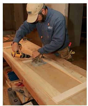
Join the frame with pocket screws. I bore two pocket holes at each stile-to-rail joint, spacing the holes about 4 in. apart along the top rail where the stool will be attached later. Before attaching the plywood back, I smooth the frame with an orbital sander.
