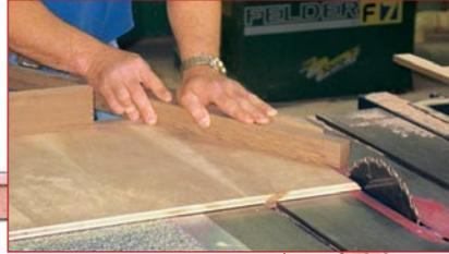
**2.** Next, I fitted a long diagonal that bisected the rectangle. Because cuts beyond 45° are difficult to handle on a miter saw, I set up a crosscut sled on the tablesaw. A temporary fence screwed to the base orients the railing stock at the correct angle.
